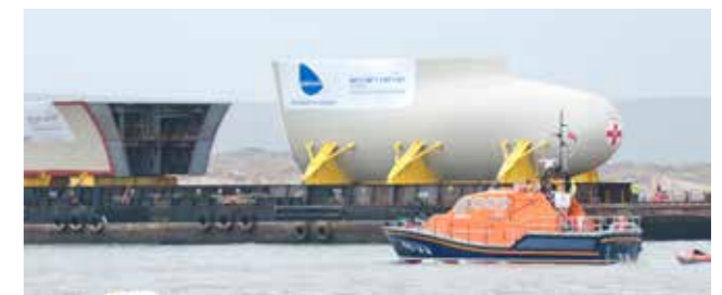
QEC aircraft carrier bow section being transported from Appledore to Rosyth
